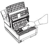
7. Remove the toner cartridge from its package and gently shake it from side to side to distribute the toner. Then
